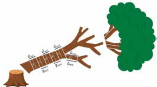
Figure 2 Schematic design of the Huber method used for destructive tree sampling. d is the measured diameter at the midpoint of each segment; L is the stem or branch length; g is the cross-sectional area.
