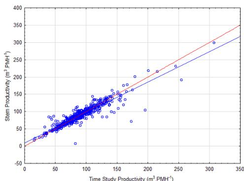
**Figure 4** Plot of Stem productivity against Time Study productivity using the pooled data from Swaths I, II, III, and IV. The red line shows  $y = x$ , blue line shows the relationship from the data.
